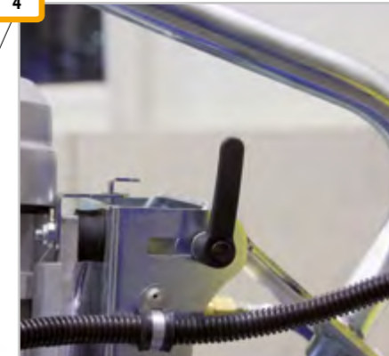
The pitch of the grinding unit needs to be adjusted. Since its pitch is infinitely variable, the grinding unit guarantees the perfect grinding angle every time.
