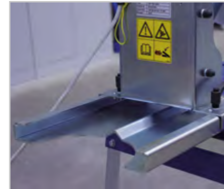
The rotary unit needs to be adjusted. The flexible positioning of the rotary unit allows for the effortless sharpening of curved blades, sporting both small and large radii.
