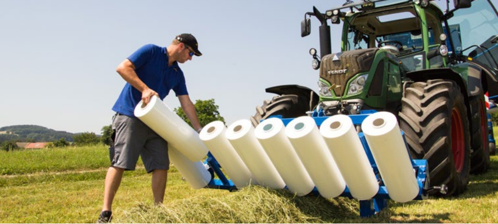
Film storage for 16 rolls of film, net or coverfilm
